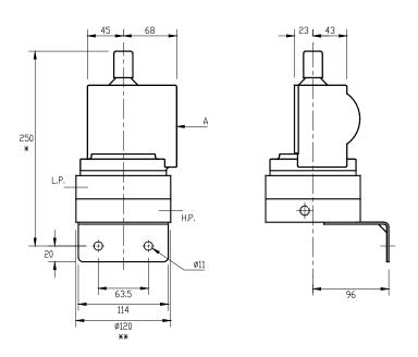
Terminal box, explosion-proof/flameproof enclosure, pneumatic valve fitted to surface 'A' \*This Dimension 260 for ½" NPT Female \*\*This Diameter 140 for ½" NPT Female L.P. - Low Pressure Connection, H.P. – High Pressure Connection
