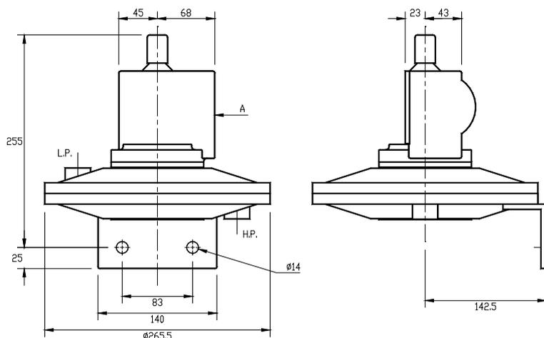
Terminal box, explosion-proof/flameproof enclosure, pneumatic valve fitted to surface 'A'
