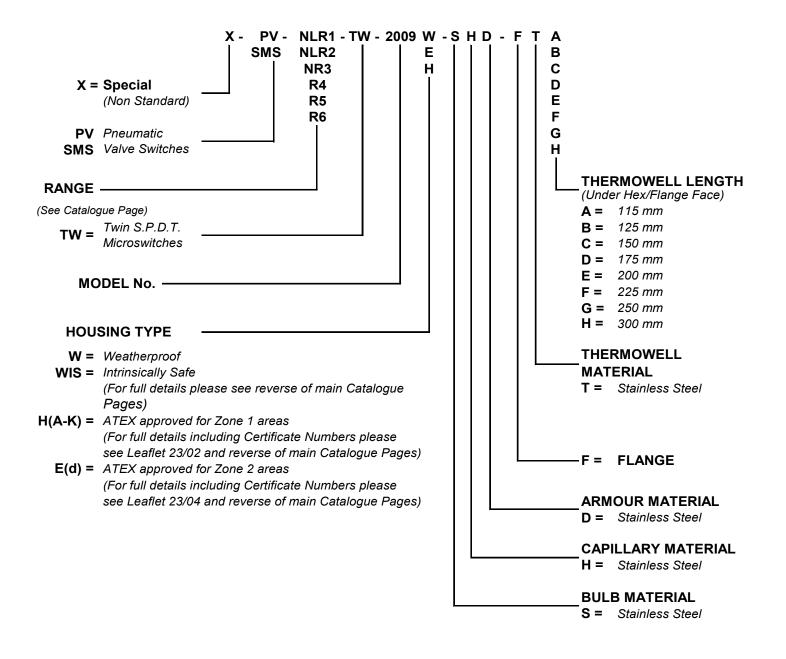
If '**Offshore**' Paint finish required, add the letters '**OS**' at the beginning of the code number, i.e.: **OS** – PV NLR1 – 2009W – SHD.
