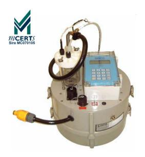
The Controller is fitted with Lithium Batteries which are used to run the Real-Time clock and to retain programme data when the unit is off.
